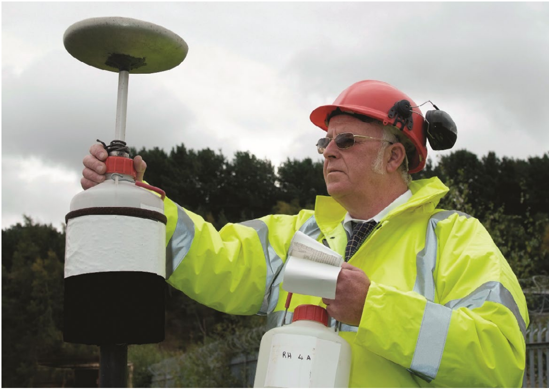
Frisbee-type dust deposit gauge used to monitor dust
