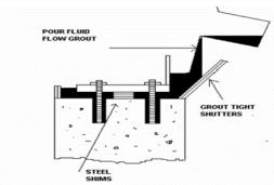
Set grout should be chamfered to ensure that unrestrained shrinkage cracking does not occur.
