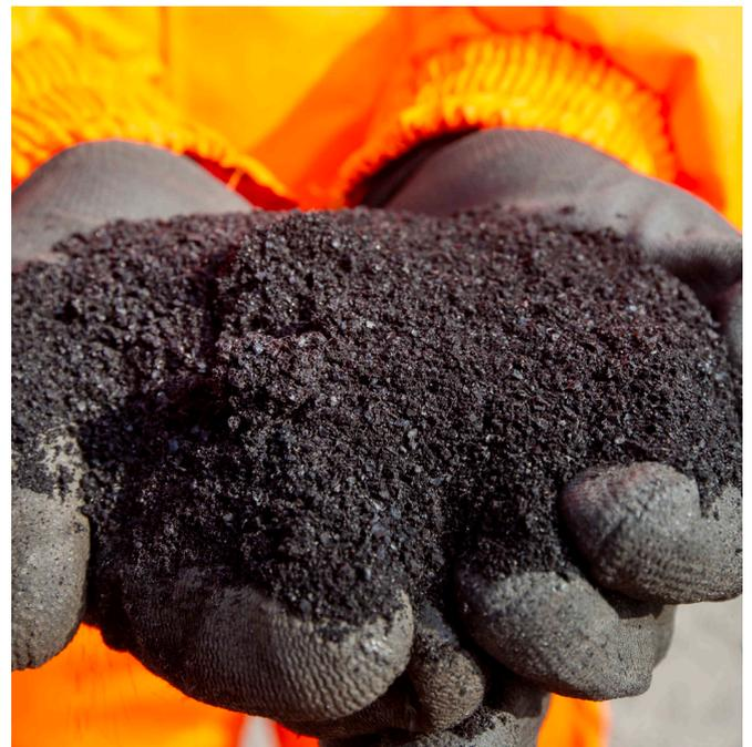
Incorporating a higher percentage of rubber modification than the asphalt mixes previously trialled with local authorities, this trial of ULTIPAVE R represented the first motorway resurfacing scheme to use an asphalt containing granulated rubber from the UK’s tyre waste stream. The UK currently exports one in four tyres, equating to 150,000 tonnes annually. Using the waste tyre stream in asphalt provides an additional disposal route in the UK.
