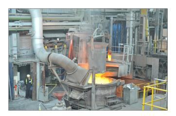
The testing of melt procedures and slag cooling offers a greater understanding of creating an end-product that could be produced on an industrial scale, with Tarmac beginning the process of testing the new clinker to understand the grinding properties and assess key performance criteria of the new material.
