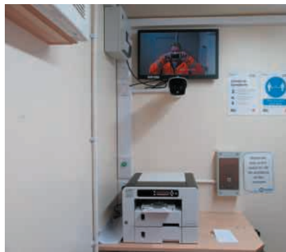
Reg Gartside, Engineering Services manager stands on the pressure mat facing the monitor. When central on the screen the thermal camera measures your temperature and takes a photograph which is then printed out along with your compliant pass for that day.
