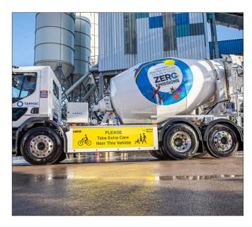
The 26 tonne Renault Trucks E-Tech D Wide comes with enhanced safety features, as the batteries provide a lower centre of gravity, improving stability. The speed of the drum rotation is also computer-controlled to optimise energy consumption for loading, unloading and transit of different types of mix.
